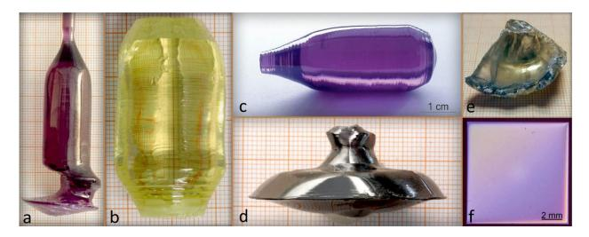
Fig. 1 Selection of some substrate crystals grown at IKZ: (a)  $(Nd,Sr)(AI,Ta)O_3$ , (b) (Mg,Zr):SrGa<sub>12</sub>O<sub>19</sub>, (c)  $(Nd,La)(Lu,Sc)O_3$ , (d) Tb<sub>2</sub>Ti<sub>2</sub>O<sub>7</sub> and (e-f) Ba<sub>2</sub>ScNbO<sub>6</sub>.
